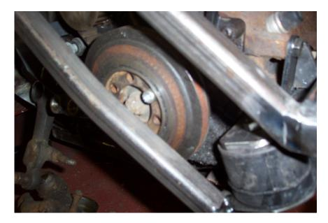
The plug head on the back of the oil filter housing needs 4mm machining off and the housing it screws into needs reducing by 7mm, ie. By sawing off ensuring the cut is square, the plug then needs refitting with a good thread sealer ie. Ptfe tape. As shown. This gives clearance to the o/s top arm pivot shaft.
