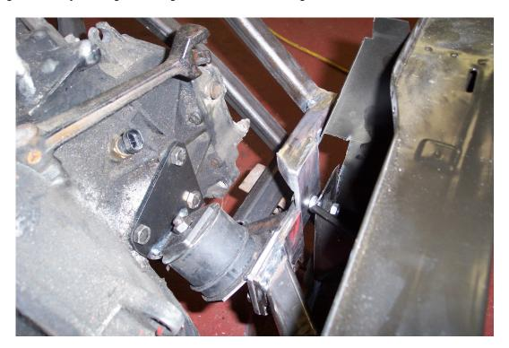
The top end can be bolted or welded to the inner wing ( welding is preferred). It is also desirable to extend the brace bars thru to the front roll cage legs for extra strength. For improved appearance new inner wings can be fabricated from the wing lip to the brace bars, this also improves the front end strength.
